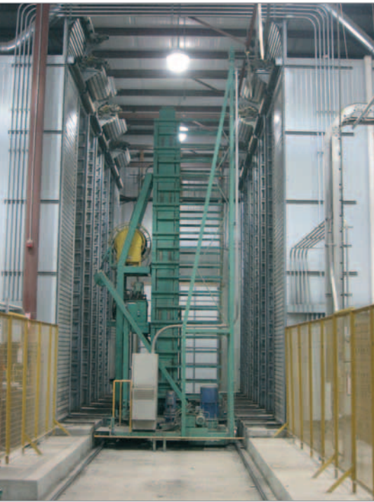
Northfield Block's transfer car that services both of Kraft Energy's Quadrix curing areas.
