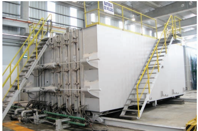
Battery Molds showing ThermalCure Circulation System to heat the molds to 55 C
