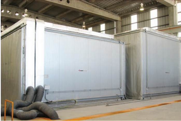
Quadrix System with Matchbox style movable curing chambers
