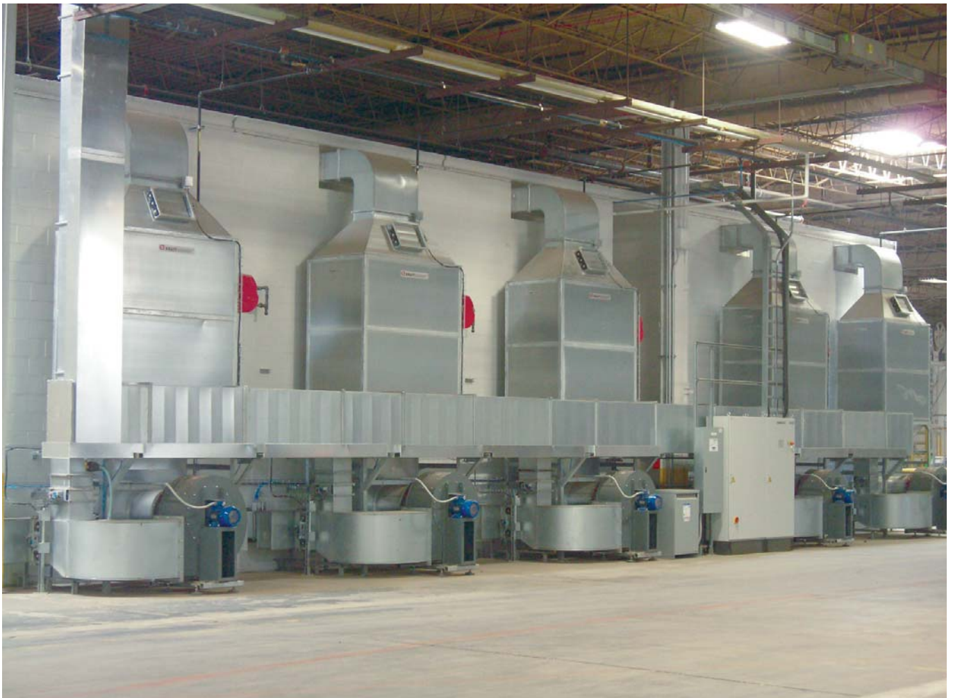
The new curing system is comprised of individual and independent Quadrix™ curing systems
