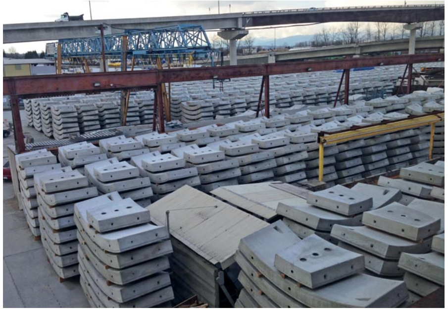
APS' Langley yard shows some of the 3504 segments/438 rings poured to date.
