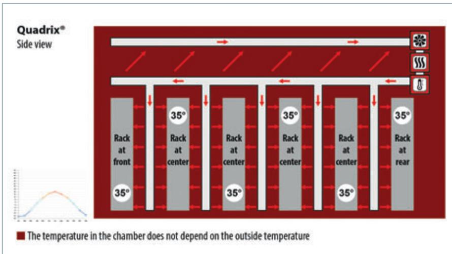
Indication of consistent temperature distribution through proper concrete curing with temperature control in a single atmosphere curing chamber.
