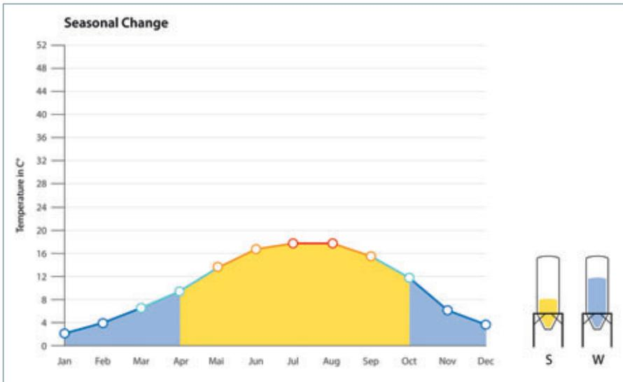
Due to seasonal changes in the ambient temperature and its affect on the speed of concrete hardening, cement content is raised/lowered in order to achieve the necessary early strength in order to cube.
