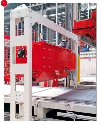
The T-REX granulate dispenser can be placed over a conveyor up to 1800mm wide.
