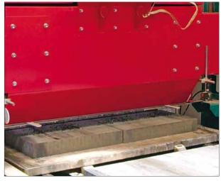
The T-REX utilizes LDPE or biodegradable granulate. While the load moves, the T-REX automatically dispenses the granulate evenly over the finished product, seperating one layer of product from the next.
