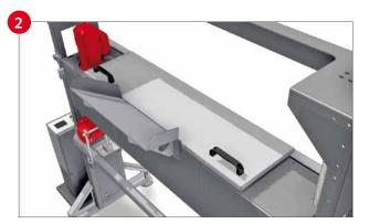
Granulate is manually filled into the hopper over a chute (optional equipment).
