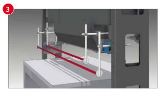
Light barriers detect transported load, initiate dispensing process and protect hopper against collision with higher load.
