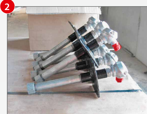
When the material temperature drops below a given set-point, the system operates automatically to provide heat to the storage bins or silos.
