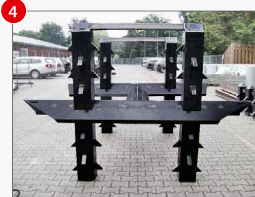
The diffuser is located at the bottom of the bin or silo – near the material discharge. A two-level diffuser is used for sand.
