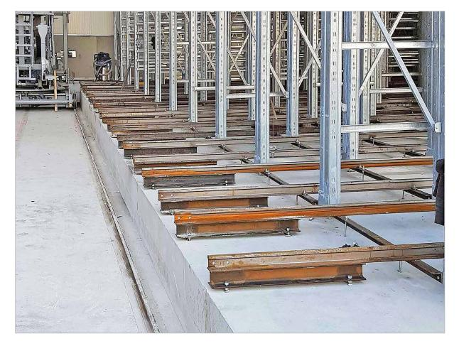
KRAFT transport rails leading into the rack come with an improved support that protects against wear-and-tear and provides for easier replacement.
