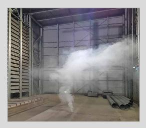
Test with smoke device shows poor air distribution in transfer car area (Competitive System)
