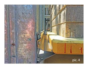
A maximum load/failure test conducted at KRAFT CURING's facilities showed no deflection of the shelve and no fastener failure with a load of more than 2 tons of concrete product per production board [picture 3]. Even combining this extreme load with an extremely uncentered board [picture 4] did not produce a failure of the system.
