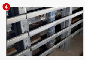
Our custom designed air distribution duct system - with air outlets located at the curing chamber floor only - guarantees the most consistent curing chamber climate distribution while maintaining a dry floor and prevention of high air velocity over the fresh concrete product surface.
