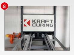
Custom-designed chamber entry and exit (letter-box style) openings - utilising warm air curtains and optional doors - prevent moist air from escaping the curing chamber into the production area. The opening frame is heated to prevent condensation from dripping on the fresh concrete product.
