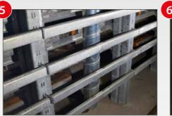
Our custom designed air distribution duct system - with air outlets located at the curing chamber floor only - guarantees the most consistent curing chamber climate distribution while maintaining a dry floor and prevention of high air velocity over the fresh concrete product surface.
