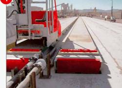
The vapor distribution system is designed using a pressure-drop algorithm and utilizes various diameter pipe and outlets in order to ensure even heat and humidity distribution. The insulated main distribution pipe outside the curing area reduces heat loss and provides a safe working environment.
