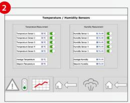
AutoCure® automatically measures and controls the curing environment. All curing data and operating status is displayed on a color display.
