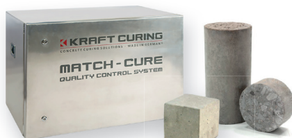
Match-Cure cures test cylinder/cubes
