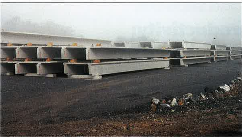
These H elements are a very popular Newcrete product and are mainly used in multi-storey car-park construction.
