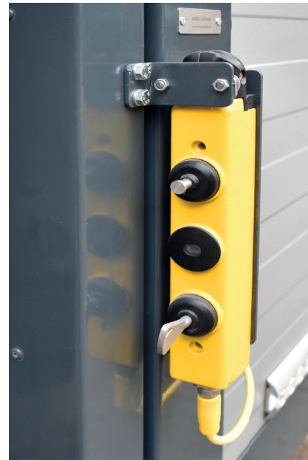
Safety Lock on curing chamber door
